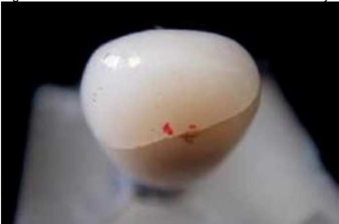
Figure 3. Cracks in metal ceramic crowns occurred at cyclic loading site.
